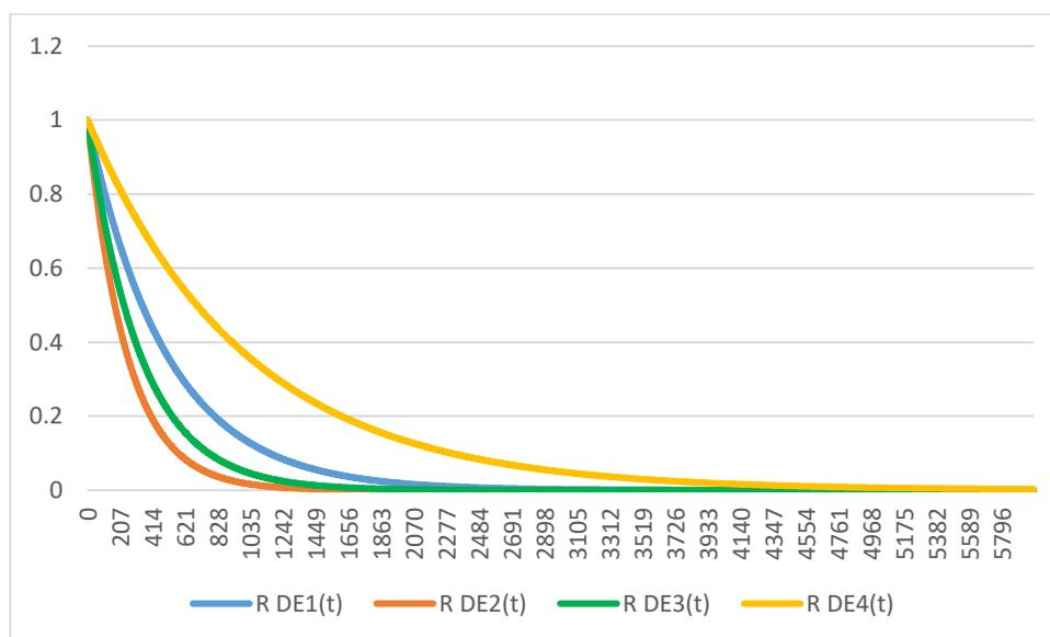
Fig (1). Main diesel engines reliability diagram
