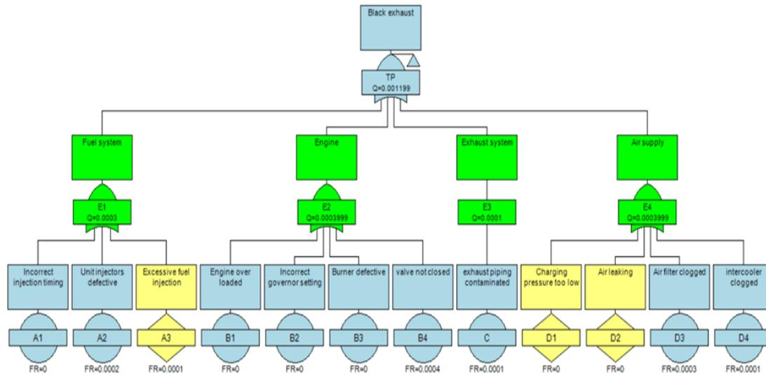
Fig (4). Black exhaust gas fault tree
