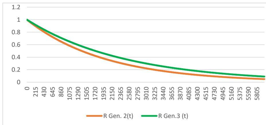
Fig (2). Reliability diagram of generator sets no.2 and 3
