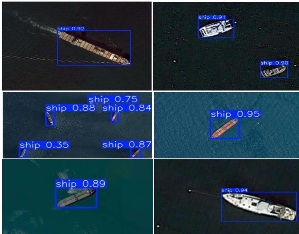
Figure 5: Results of ship detection for unseen images
